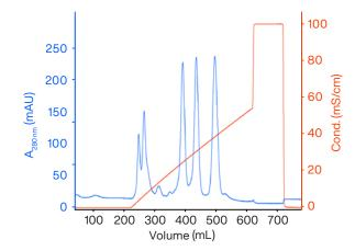
Figure 6. Separation using cation exchange chromatography. Peaks from left to right, concanavalin A,  $\alpha$ -chymotrypsinogen A, ribonuclease A and lysozyme. 4.6 mL sample applied on GoBio Prep 16x100 40S. The blue trace corresponds to absorbance at 280 nm and the red line to conductivity.
