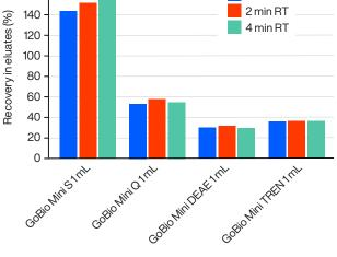
**Figure 8.** Dynamic binding capacity determined at 10% breakthrough for a 39 aa-long peptide at different residence times. The residence times used are specified in the graph.
