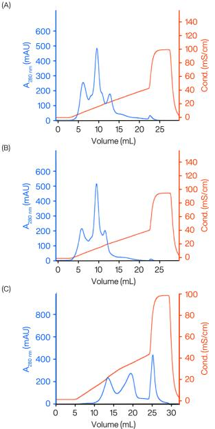
**Figure 3.** Separation using anion exchange chromatography. Peaks from left to right, apo-transferrin,  $\alpha$ -lactalbumin and soybean trypsin inhibitor. (A) 2 mL sample on GoBio Mini Q 1 mL, (B) 2.5 mL sample on GoBio Mini DEAE 1 mL, (C) 2.5 mL sample on GoBio Mini TREN 1 mL. The blue line corresponds to absorbance at 280 nm and the red line to conductivity.
