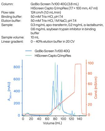
**Figure 5.** Separation of acidic proteins using anion exchange chromatography. Peaks from left to right, apo-transferrin,  $\alpha$ -lactalbumin and soybean trypsin inhibitor. 10 mL sample onto GoBio Screen 7x100 40Q and HiScreen Capto Q ImpRes. The blue and green traces correspond to absorbance at 280 nm and the red line to conductivity.
