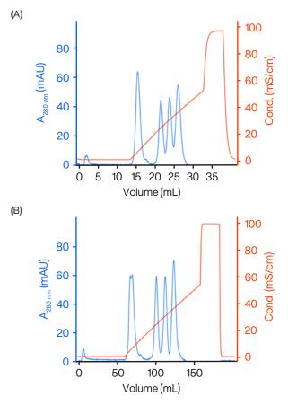
Figure 2. Separation using cation exchange chromatography. Peaks from left to right, concanavalin A,  $\alpha$ -chymotrypsinogen A, ribonuclease A and lysozyme. (A) 0.25 mL sample applied onto GoBio Mini S 1 mL and (B) 1.25 mL sample applied onto GoBio Mini S 5 mL. The blue line corresponds to absorbance at 280 nm and the red line to conductivity.
