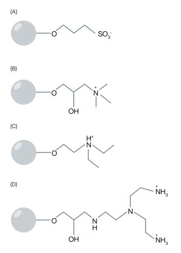
Figure 1. Structure of the ligand used in (A) WorkBeads 40S, (B) WorkBeads 40Q, (C) WorkBeads 40 DEAE and (D) WorkBeads 40 TREN.
