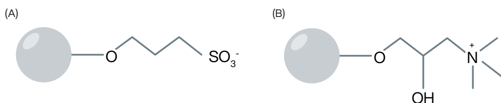
Figure 1. Structure of the ligand used in WorkBeads 40S (A) and WorkBeads 40Q (B).
