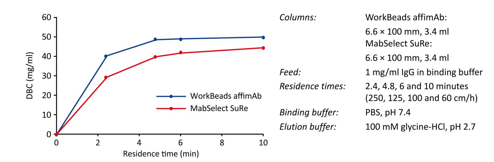
Figure 1. DBC for human polyclonal IgG determined at different flow rates (residence times) by frontal analysis on WorkBeads affimAb (blue) and MabSelect SuRe (red).
