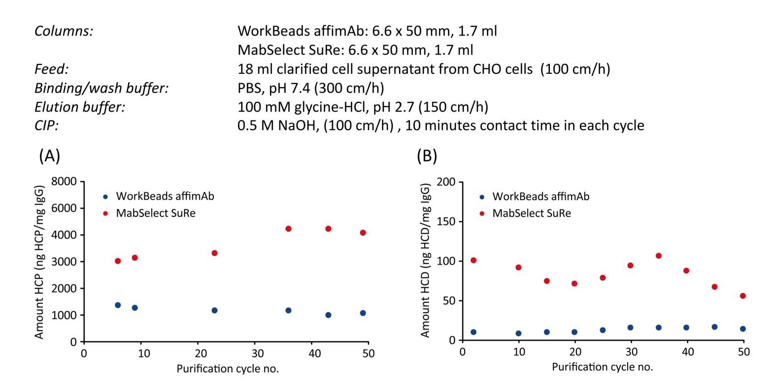
Figure 3. Comparison of residual HCP (A) and HCD (B) in mAb eluates from WorkBeads affimAb and MabSelect SuRe during 50 purification cycles.
