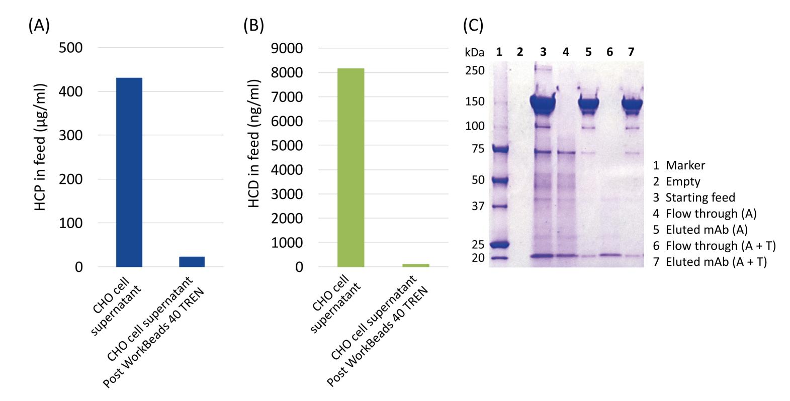
Figure 4. Levels of impurities in CHO cell supernatant before and after WorkBeads 40 TREN treatment. (A) HCP and (B) HCD in mAb sample loaded onto the protein A resin. (C) SDS-PAGE analyses of the feed, flow-through and eluted mAb, with or without WorkBeads 40 TREN (T) upstream WorkBeads affimAb (A).
