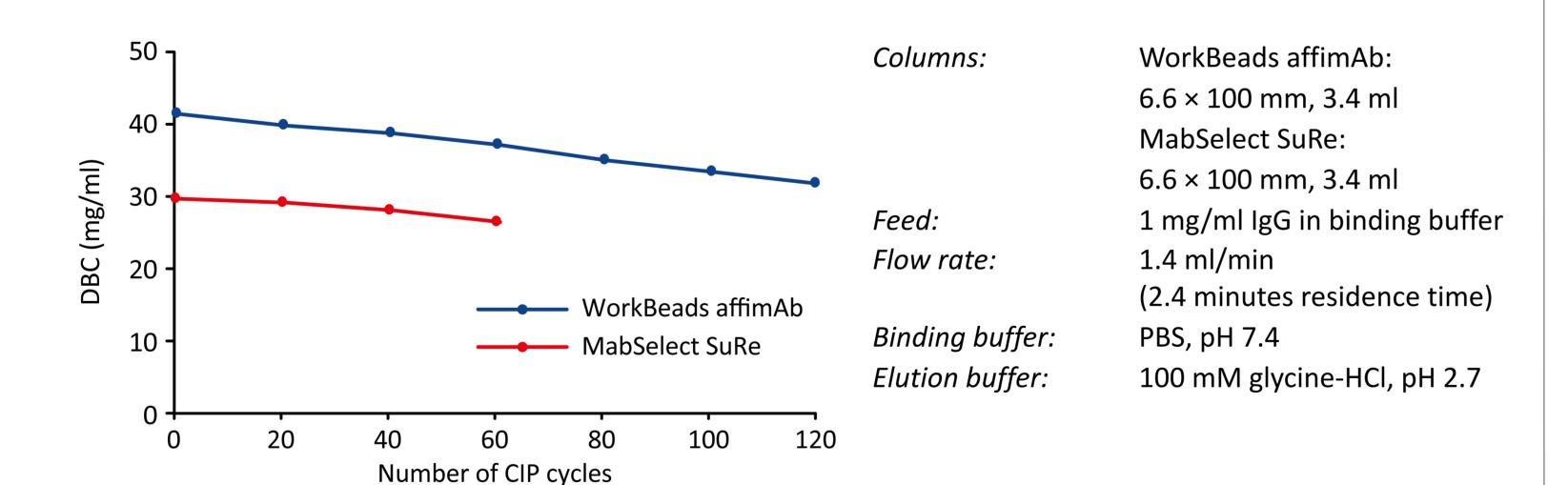
Figure 2. DBC determined with polyclonal human IgG at 2.4 minutes residence time.  $Q_{B10\%}$  measured at every 20<sup>th</sup> CIP cycle for WorkBeads affimAb and MabSelect SuRe.
