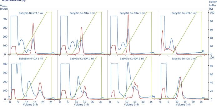
Figure 2. Comparison of purifications of His<sub>6</sub>-GFP on BabyBio NTA 1 ml and BabyBio IDA 1 ml charged with Ni<sup>2+</sup>, Co<sup>2+</sup>, Cu<sup>2+</sup> and Zn<sup>2+</sup>. Blue line: absorbance, 280 nm. Red line: absorbance, 490 nm (specific for His<sub>6</sub>-GFP). Green line: % elution buffer.
